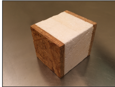
Photo #3: Common SIPS panel design
